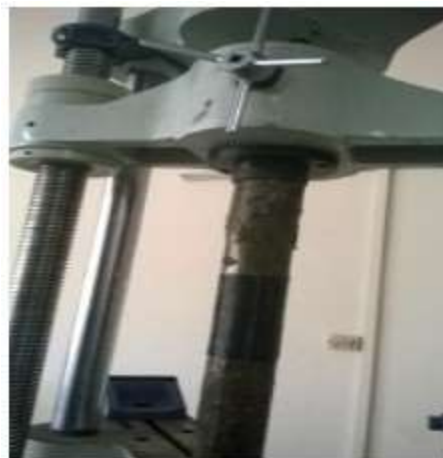
Fig 2. Compression Test on Specimen (Retrofitted at Center)
